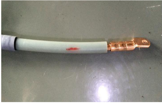
Figure 4: Defect model of cable insulation scratch.
